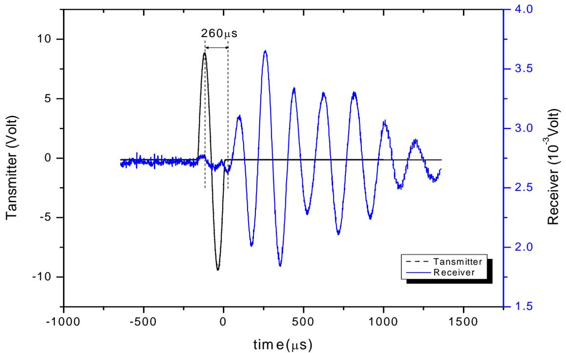
**Fig.6** Typical P wave signals recorded on oscilloscope for soaked sample
