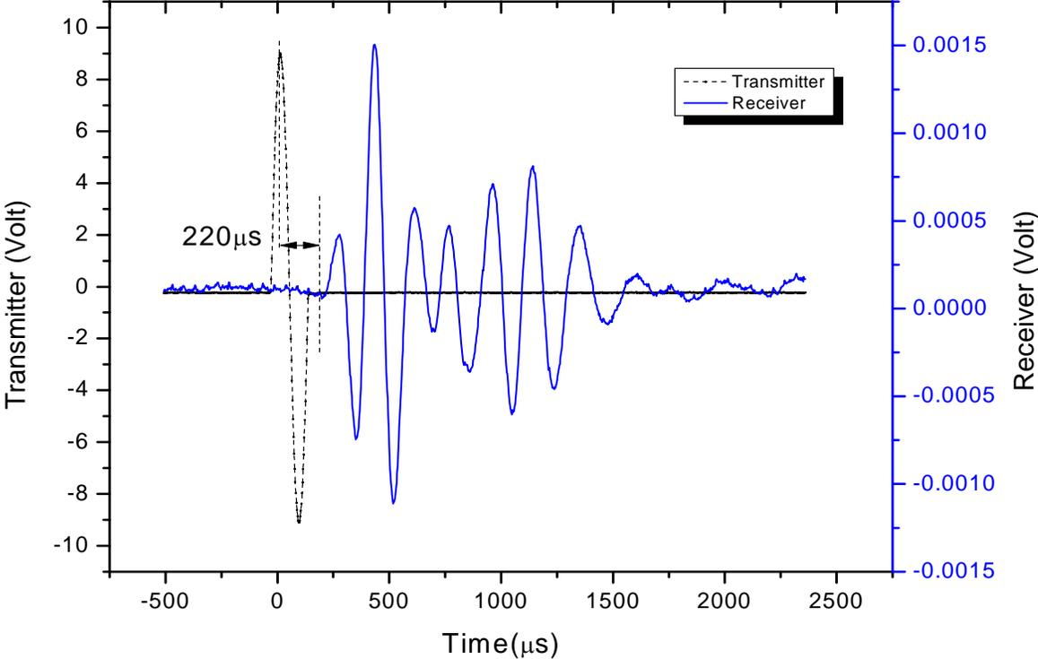
**Fig.8 Typical P wave signals recorded on oscilloscope for unsoaked sample**
