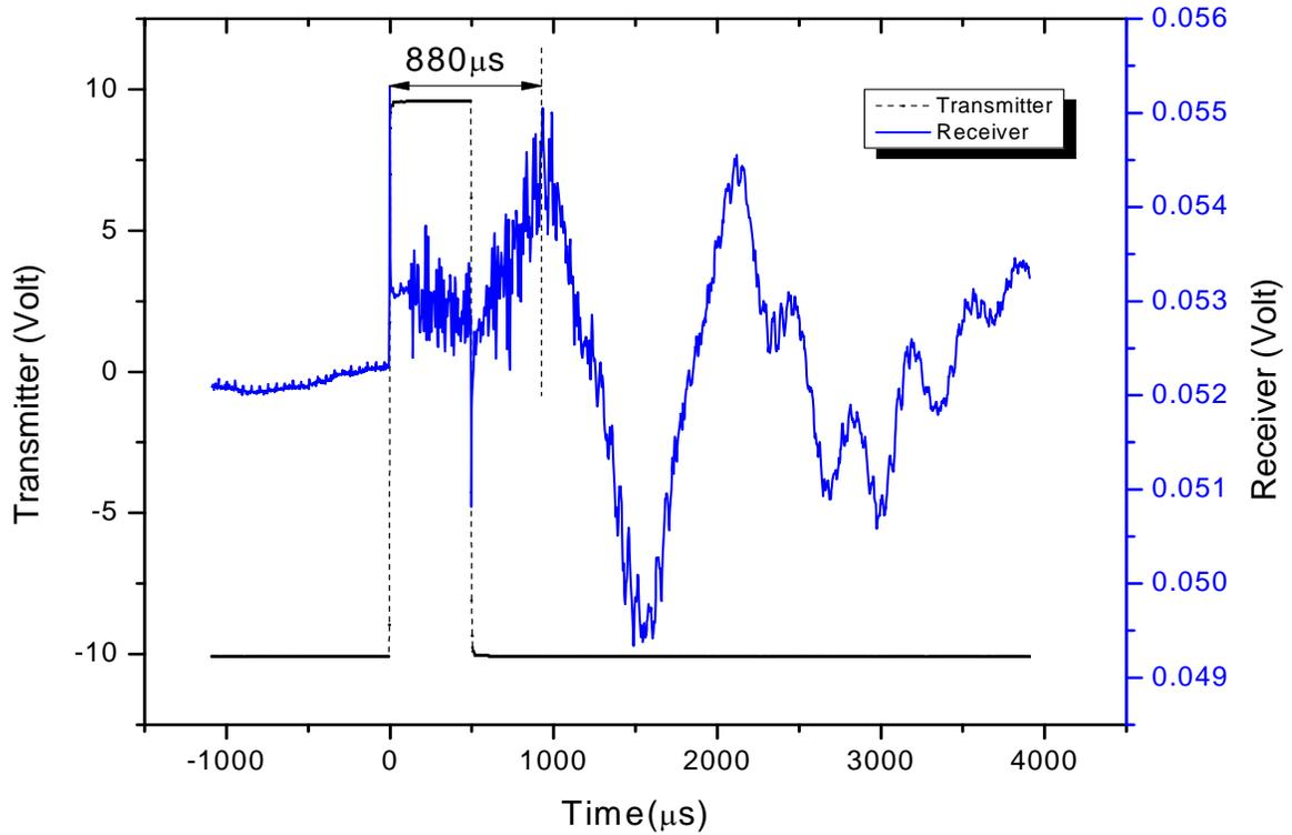
**Fig.9 Typical S wave signals recorded on oscilloscope for unsoaked sample**
