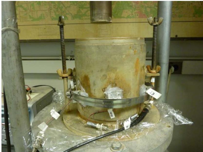
**Fig.4 Bender and Extender Element Test Set-up**
