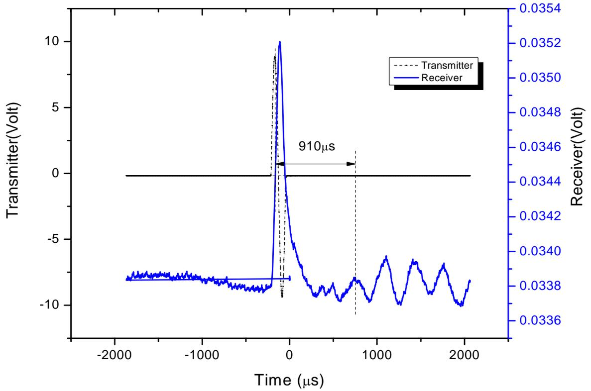
**Fig.7 Typical S wave signals recorded on oscilloscope for soaked sample**
