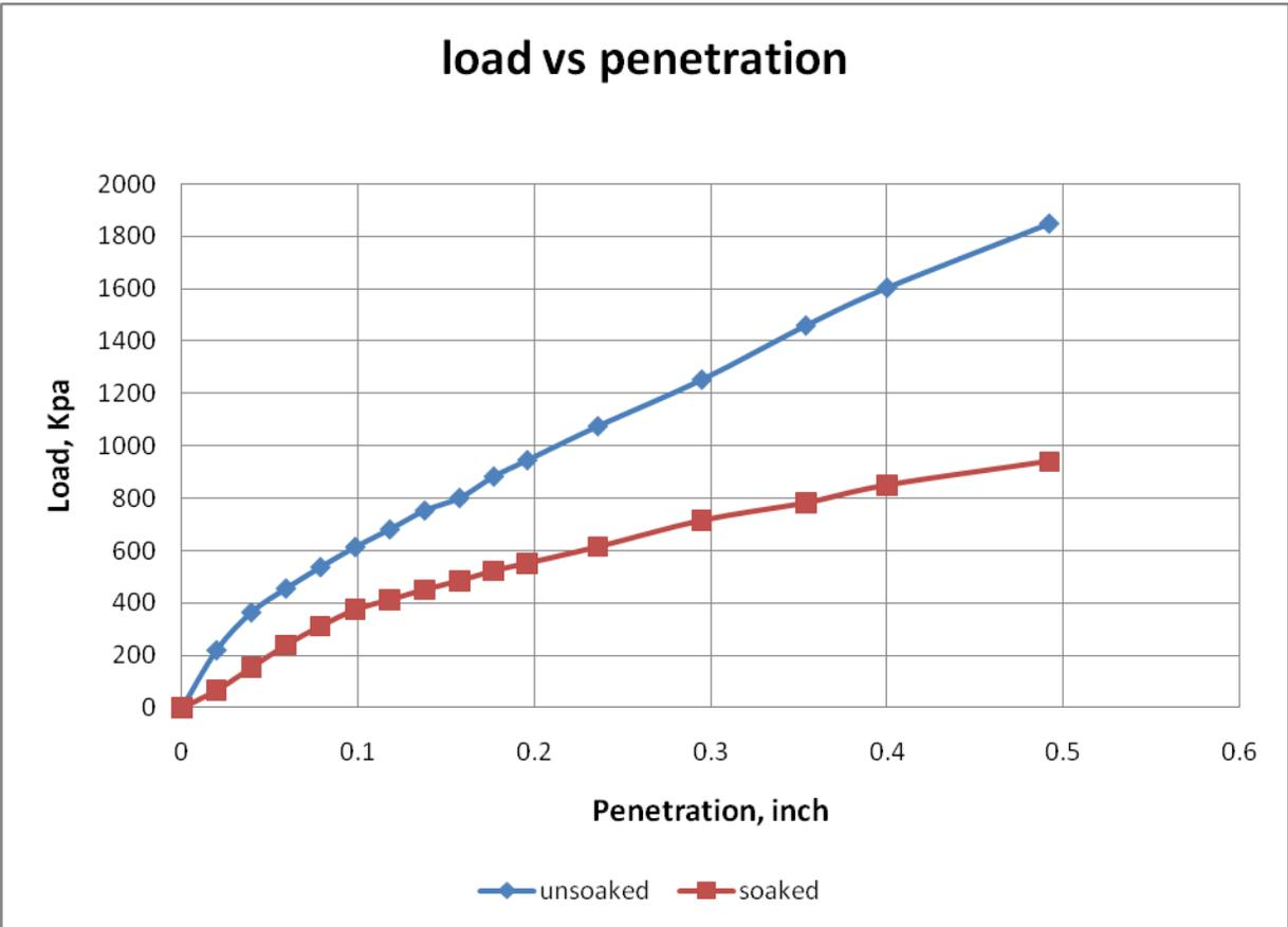
**Figure 3 Results of CBR tests on the clay**
