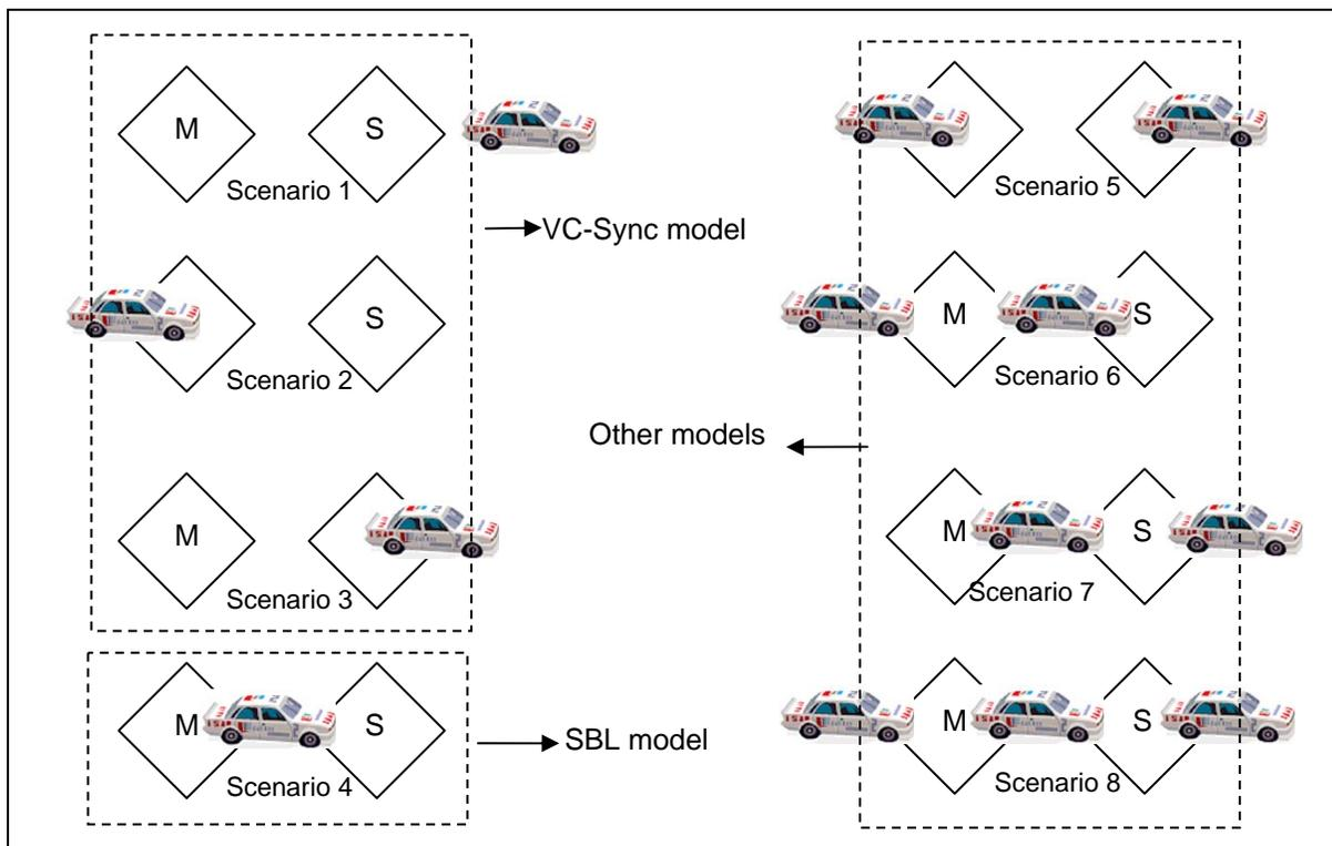
**Figure 1. Eight Scenarios of Vehicle Stopping on Loops under Stop-and-go Flow**
